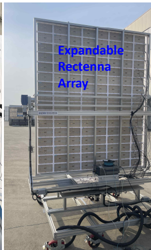
Modular Microwave Power Beaming System
